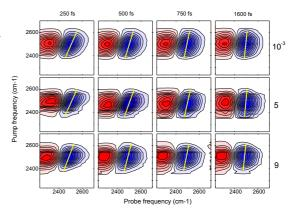
value of 1. 3 ps. On the other hand, we observe only a moderate decrease (1.7 to 1.4 ps) of the picosecond component of spectral diffusion ( $\tau_{SD}$ ) at 298 K in the inspected pressure range. In the second phase of our project we study the dynamical exchange process between "differently bounded" water molecules in a 5M solution of ClO<sub>4</sub><sup>-</sup> as a function of pressure.
